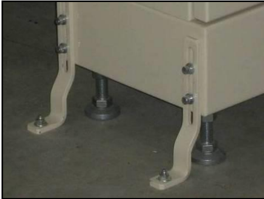
Floor-mounted manufacturing equipment anchorage
