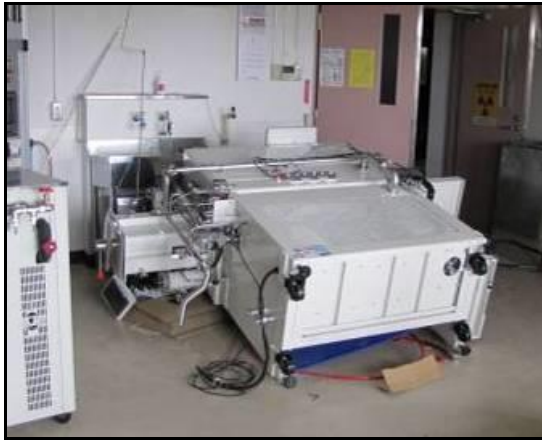
Topped unrestrained lab workstations (2011 M9.0 Japan earthquake)
